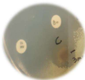
Figure 8. Representative inhibition zone of A70:K30 hydrogel scaffold with 5% extract against S. aureus .
